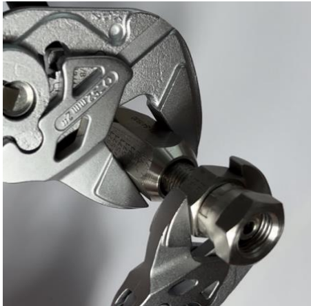
Illustration 13 - Hold on to the socket while screwing in the nipple
