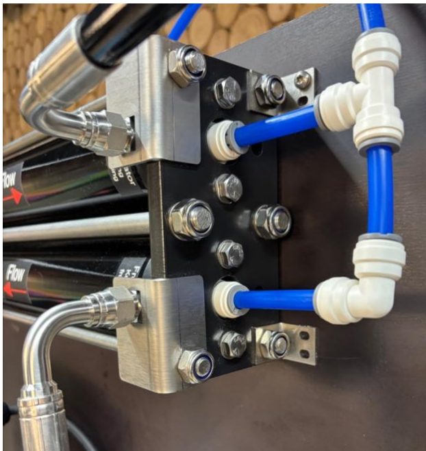
Illustration 10 – Membrane unit with connections for sea water and product water
