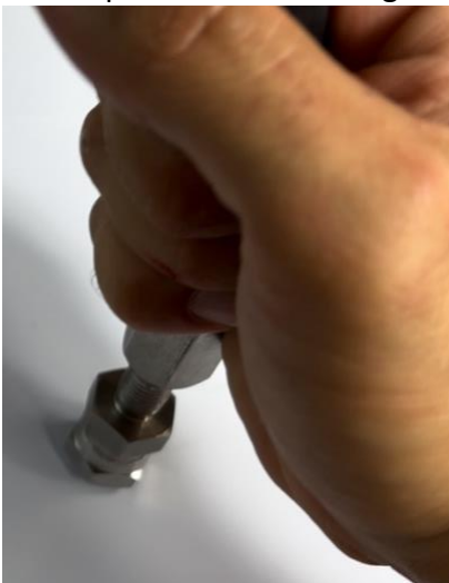
Illustration 13 - Pressing the nipple into the hose with pre-assembled socket
