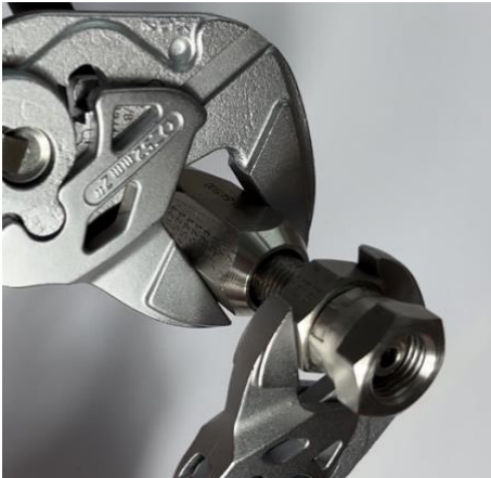
Illustration 14 - Hold on to the socket while screwing in the nipple
