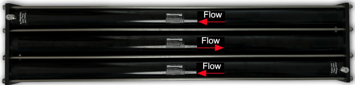
Illustration 2 - Mounting direction membrane in pressure vessel
