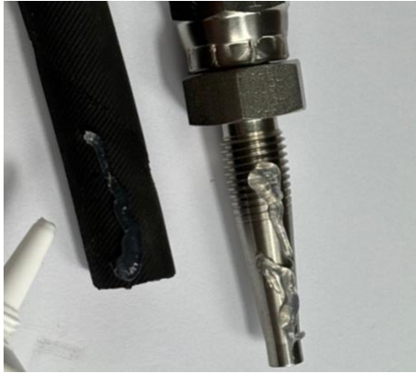
Illustration 10 - Silicone grease-coated sheath and nipple
