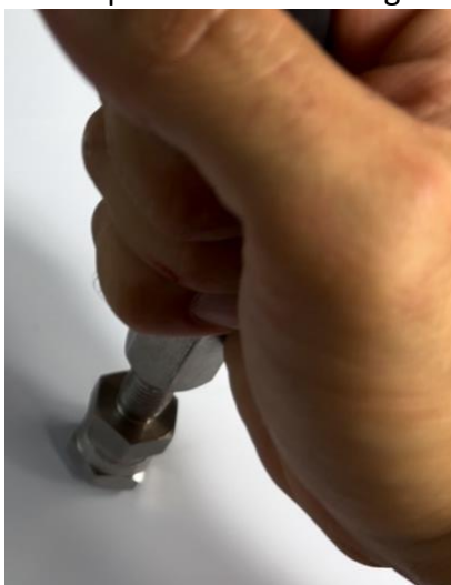
Illustration 12 - Pressing the nipple into the hose with pre-assembled socket
