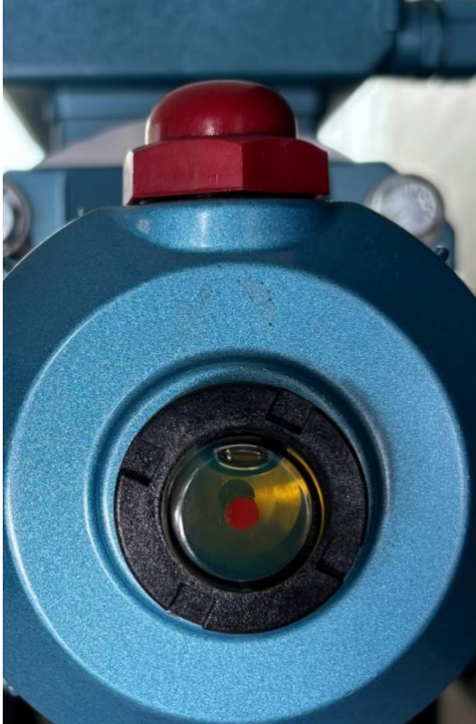
Illustration 6 - Oil level above the red marker for the minimum level.
