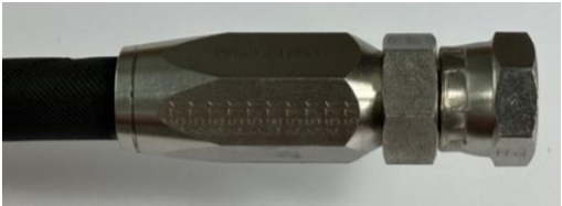
Illustration 14 - Correctly mounted screw fitting - socket and nipple are fully screwed together
