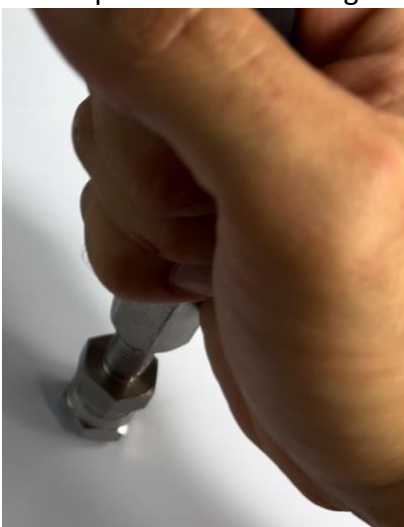
Illustration 11 - Pressing the nipple into the hose with pre-assembled socket
