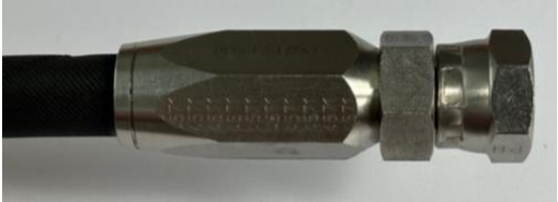
Illustration 13 - Correctly mounted screw fitting - socket and nipple are fully screwed together
