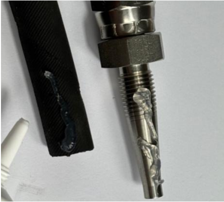
Illustration 8 - Silicone grease-coated sheath and nipple
