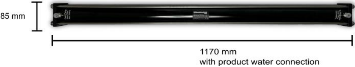
Illustration 16 - Dimensions membrane unit 1x2540
